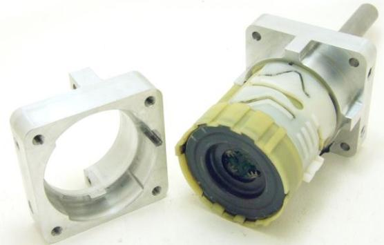
The transmission only fits into the rear transmission mount in one orientation. Line up the notch on the rear transmission mount with the protrusion on the side of the transmission.
