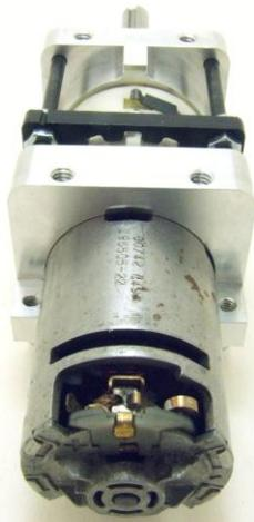
With the crimps adjusted, slide the motor into the rear transmission mount. Rotate the motor slightly to engage the planetary gears. Push in the motor until the forward case vents are barely flush with the face of the rear transmission mount, as shown. The motor can be installed in any orientation.
