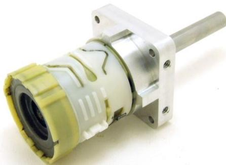
Gently push the transmission into the output assembly while rotating the output shaft with your hand to line up the output spline with the 5-sided output socket.
