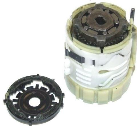
Remove the black plastic front cover from the 397892 transmission by gently bending the two clips molded into the casing. The five anti-backdrive roller pins and 5-sided output coupler will be visible.
