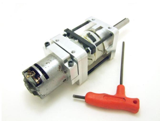
Finally, install the motor clamp ring and the two #10-24 x 1.5" screws using a 5/32" hex wrench. Take care to tighten the screws evenly, and do not exceed more than  $\frac{1}{4}$  turn per screw from a hand-tight position. When fully tightened, the gap between the motor clamp ring and the transmission mount is approximately 0.025".
