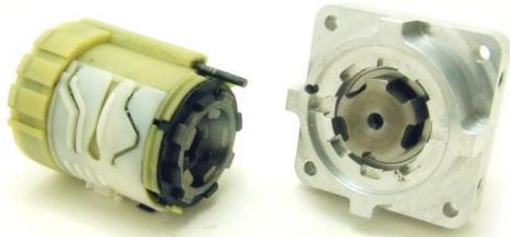
The transmission only fits into the output assembly in one orientation. Use the torque clutch adjustment plunger to align the transmission.
