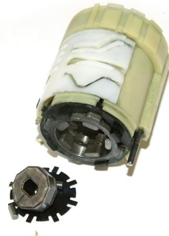
Remove and discard the roller pins, the 5-sided output coupler, and the black steel shim. Reinstall the black plastic cover in the same orientation it was removed from. After this step, the output of the transmission will be a 5-sided socket.
