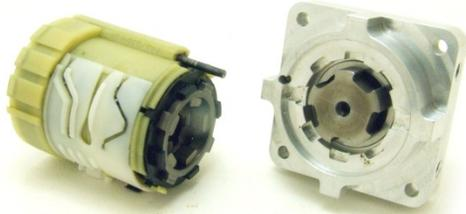
The transmission only fits into the output assembly in one orientation. Use the torque clutch adjustment plunger to align the transmission.
