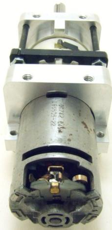
**(Note: Motor shown with v1.0 gear selector retainer)** Slide the motor into the rear transmission mount, rotating slightly to engage the planetary gears. Push in the motor until the forward case vents are barely flush with the face of the rear transmission mount, as shown. The motor can be installed in any orientation otherwise.
