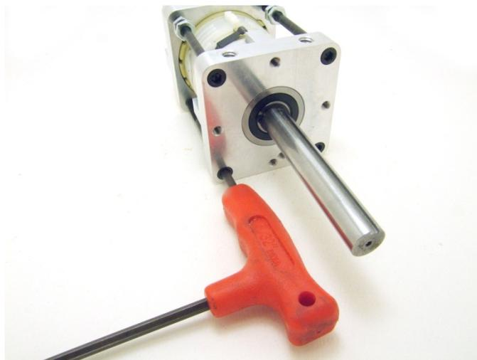
Use a 5/32" hex wrench to tighten the face mounting screws. To maintain squareness, do not tighten one screw "all the way" first.
